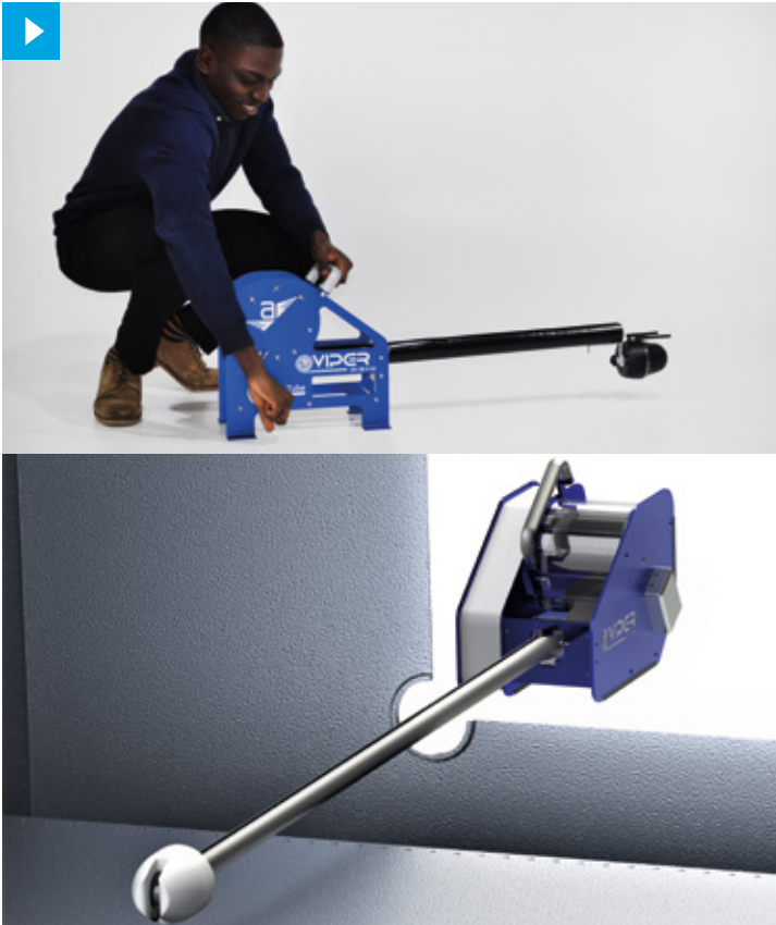
VIPER – REMOTE DEPLOYMENT SYSTEM USING BISTABLE REELED COMPOSITE.
