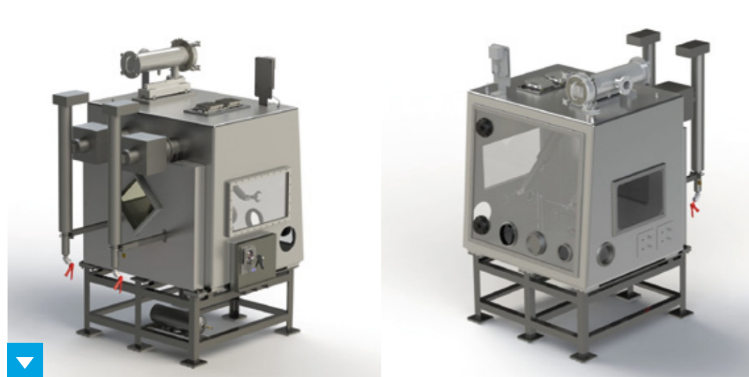
AQUILA MULTI-FUNCTIONAL CELL USED FOR INACTIVE REMOTE HANDLING TRIALS.
